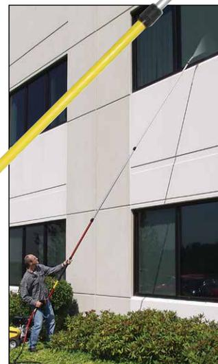
Telescoping lances offer a safe alternative to pressure washing with a ladder or scaffolding
